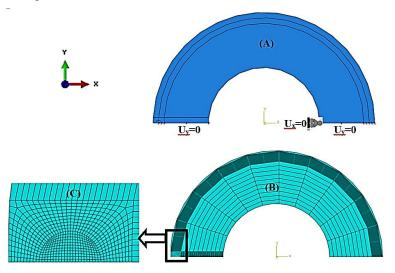
Figure 2. FE model of cracked Hollow cylinder: (a) bondoury conditions; (b) model and typical mesh; (c) mesh around the crack tip.
