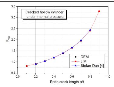
Figure 3. Variation of Knor versus the crack length.
