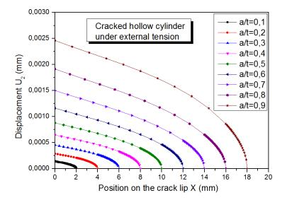
Figure 9. Variation of displacements of the crack surface for different lengths of cracks.
