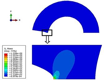
Figure 4. ISO- image of the stress distributions in the vicinity of the crack lenth a=18mm
