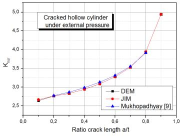
Figure 7. Variation of  $K_{nor}$  versus the crack length
