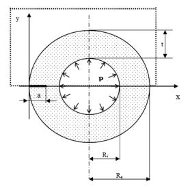
Figure 1. Geometrical model [6].
