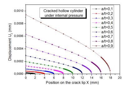
Figure 5. Variation of displacements of the crack surface for different lengths of cracks
