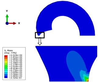
Figure 8. ISO- image of the stress distributions in the vicinity of the crack lenth a=18mm
