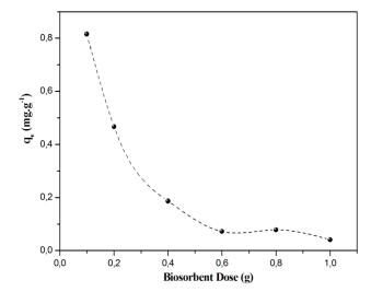
Figure 2. Effect of biosorbent dose on the adsorption capacity of MB.
