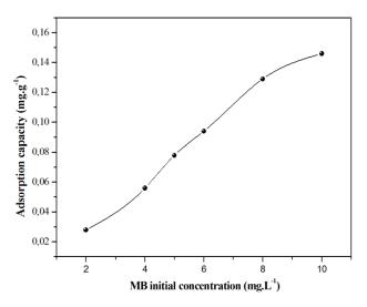
Figure 1. Effect of initial MB concentration on the adsorption capacity of prepared biosorbent.
