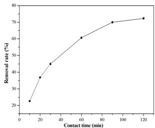
Figure 3. Effect of contact time on the adsorption of MB by prepared biosorbent.
