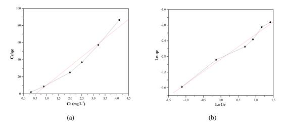
Figure 4. Langmuir isotherm of MB on the prepared biosorbent (a), Freundlich isotherm of MB on the prepared biosorbent (b)
